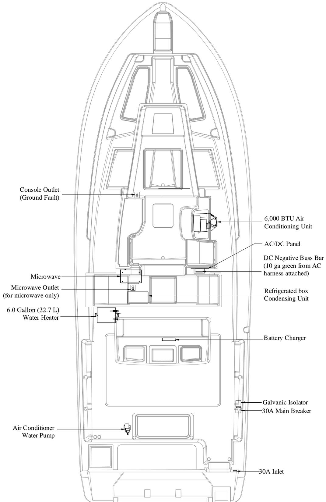
120 Volt AC Wiring One-Line Diagram
