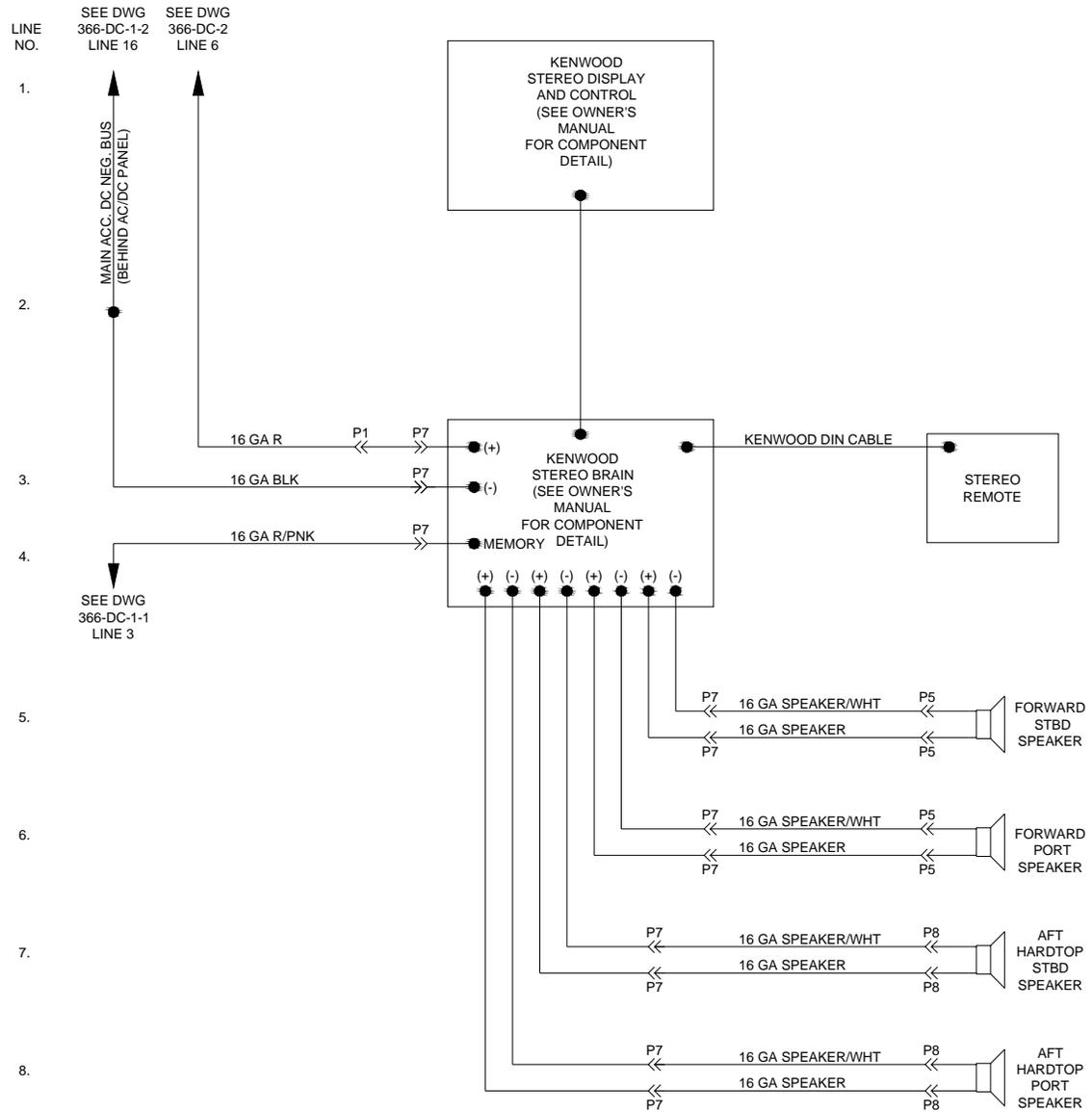
12 Volt DC Stereo Diagram with Satellite Radio
